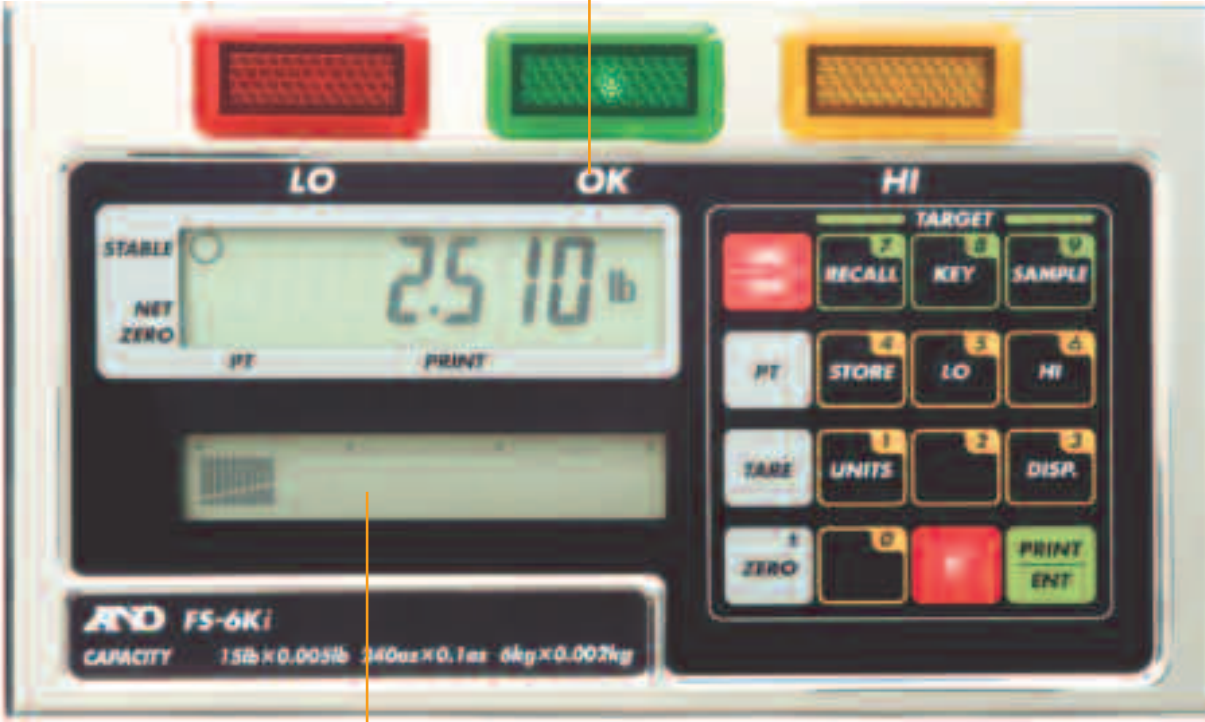
Analog Sweep Display for Target Weighings
